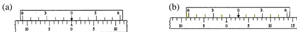
Figure 4. (a) Extended vernier, (b) measuring the length using an extended vernier scale (note the arrow)
