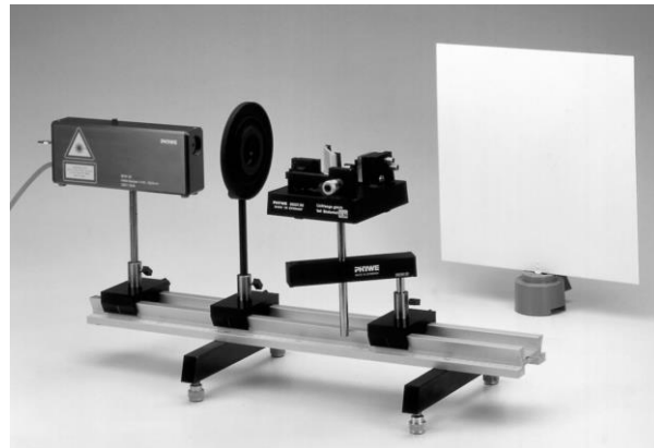
Fig. 6: Experimental set-up for measuring wavelengths with the Michelson interferometer.
